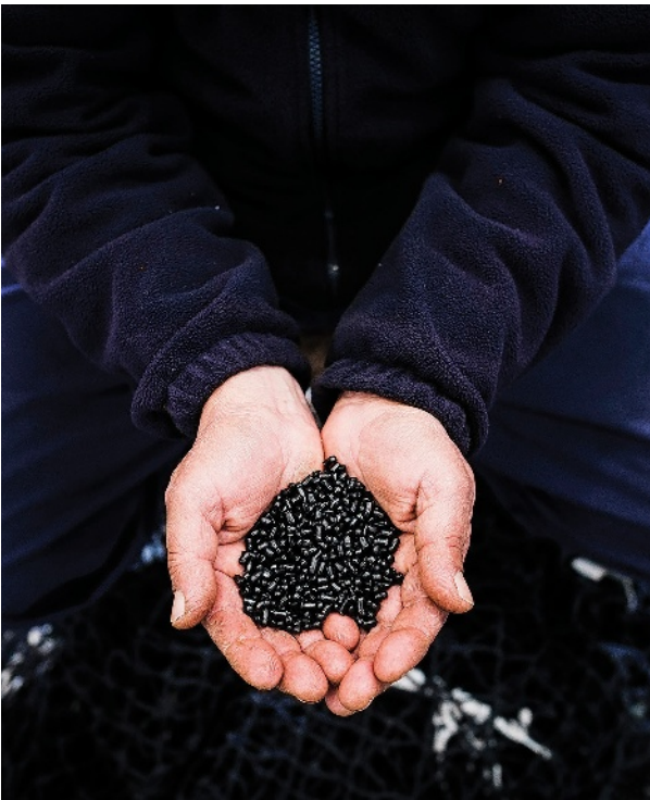
Bureo trains and employs teams of local community members to process the collected nets and turn them into a raw material source. (Image: Alfred Jürgen Westermeyer)
