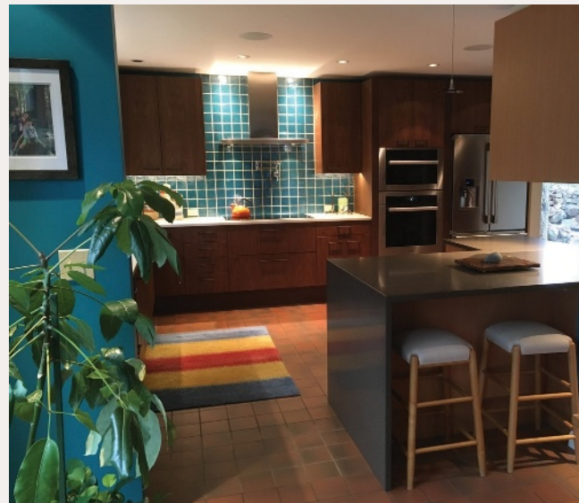
Kitchen by Bonneville Design includes features such as a convertible cook top, sink base cabinetry that pulls out for knee space, and clear paths of travel with full turning radius in the center to accommodate aging-in-place. (Image: Bonneville Design)
